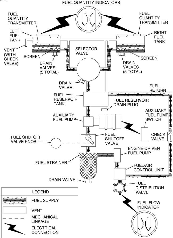
Figure 7-6. Fuel System Schematic
