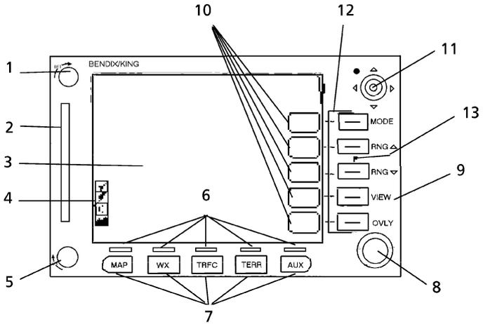
1. BRIGHTNESS CONTROL -- Clockwise rotation will increase the brightness of the display. Counter-clockwise rotation decreases the display brightness.
