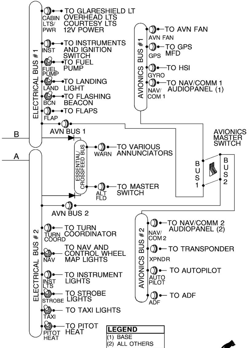
Figure 7-7A. Electrical Schematic (Serials 172S8704 and On)
