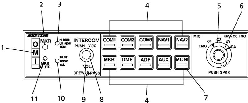
1. MARKER BEACON ANNUNCIATOR LIGHTS -- The three-light marker beacon receiver built into the KMA 26 gives a visual and aural signal when the ship's antenna passes over a 75 MHz beacon. The blue, amber, and white lights on the faceplate, as well as the audio tones, identify the beacon type.
