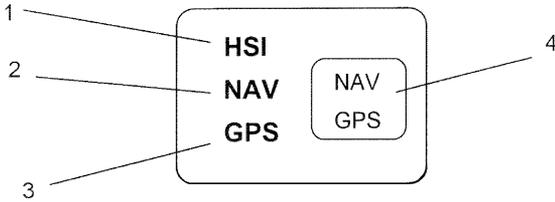
1. HSI ANNUNCIATOR LIGHT -- This label is present when the optional HSI is installed. The HSI course pointer provides course datum to the autopilot.
